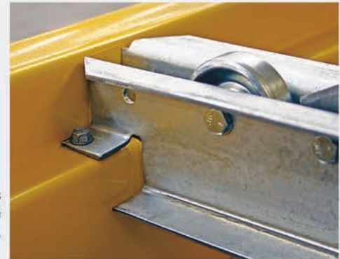
Metal skate wheel rails are notched to fit into the step of pallet rack beams.
