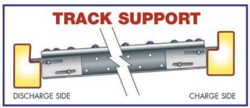
Slotted end supports adjust to vary length and ensure proper fit
