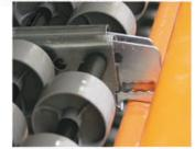
CHARGE END Heavy-duty end bracket rests in step of beam and adjusts incermentally.
