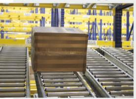
Full-width box support helps provide flow for damaged boxes.
