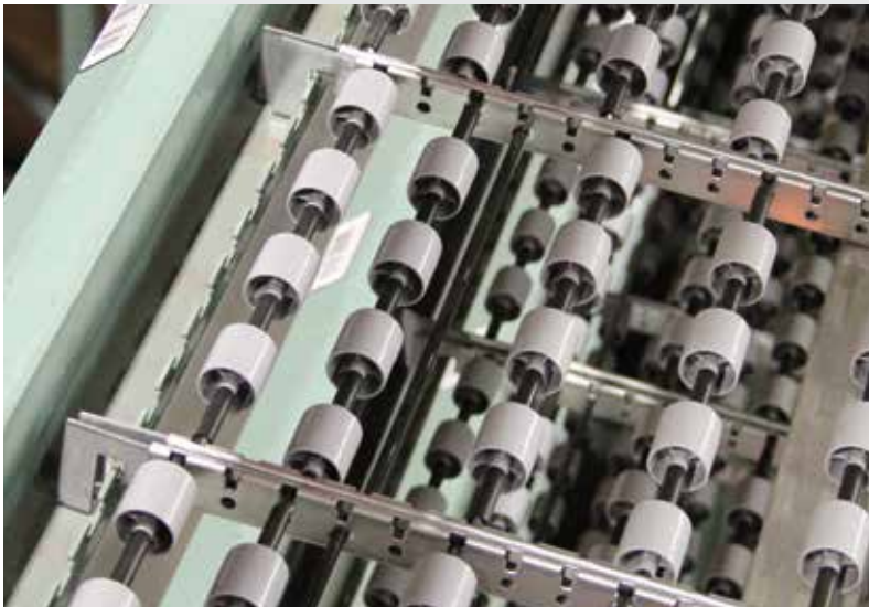
Entry and exit brackets mount into carton flow shelf members with no loss of clearance and no labeling disruption.
