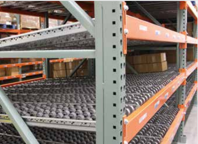
Contiguous wheel span creates a deck for mixed package width on the same shelf maximizing space and efficiency.
