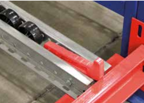
Solid metal pallet stops are integrated into every lane.
